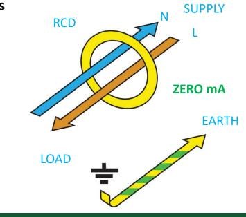
If there is an earth fault the neutral current will be lower than the line current. This imbalance produces an output from the current transformer which is used to trip the RCD and so break the circuit
