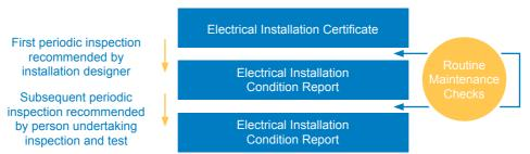
All documentation associated with the electrical installation should be kept safely and be available as evidence of ongoing maintenance.
