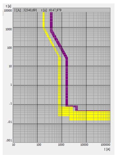
Figure 8 - Two different moulded case circuit breakers modelled in 'designgenie' to obtain a discrimination analysis
